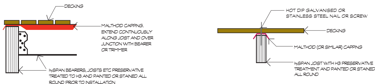
FIGURE 2 DETAILS FOR WEATHER EXPOSED DECKS
